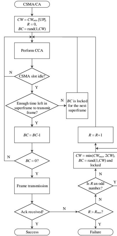
Fig. 2. IEEE 802.15.6 CSMA/CA mechanism. In this figure “Y”, “N” and UP stands for “Yes”, “No” and user priority, respectively.
