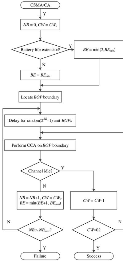
Fig. 1. IEEE 802.15.4 CSMA/CA mechanism. In this figure “Y” and “N” stands for “Yes” and “No”, respectively.
